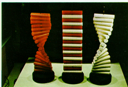
Fig. 2. Right and left-handed screws representing the minimum energy configuration in the cholesteric mesophase (the 2 external piles represent enantiomeric structures, the central one a compensated structure).
