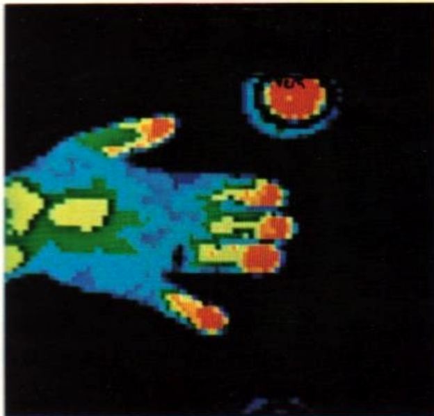
Computer processed thermogram of the hand recorded from a video display monitor. (Isotherms: 0.5^{\circ}\text{C} ; reference: 34^{\circ}\text{C} ).
