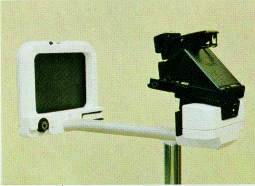
Fig. 20A-B Documentation of the C.T. image. A) Photographic system on slides; B) Polaroid system. There is fixed distance between the recording system focus and the plate. The light source for the documentation is obtained by an incorporated flash
